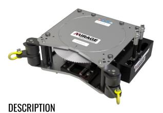
The MBS 1360 bolt saw is designed to clamp onto flanges and cut the studs through the flange gap. The pivoting clamps and ratchet strap ensures a single machine can be mounted onto a wide range of flange diameters
